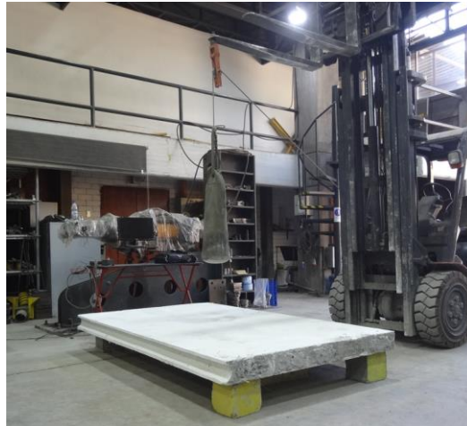
Photograph 7.4.1.1. General view of the setup of the panel subjected to the impact test.
