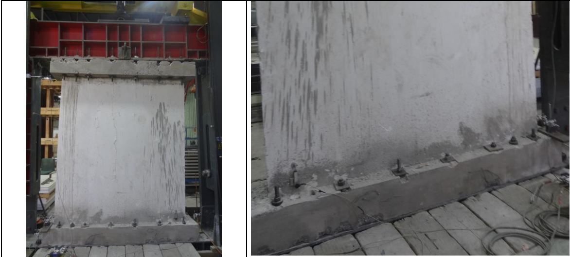
Photograph 7.2.1.1. General view of the horizontal load (shear) test setup.
