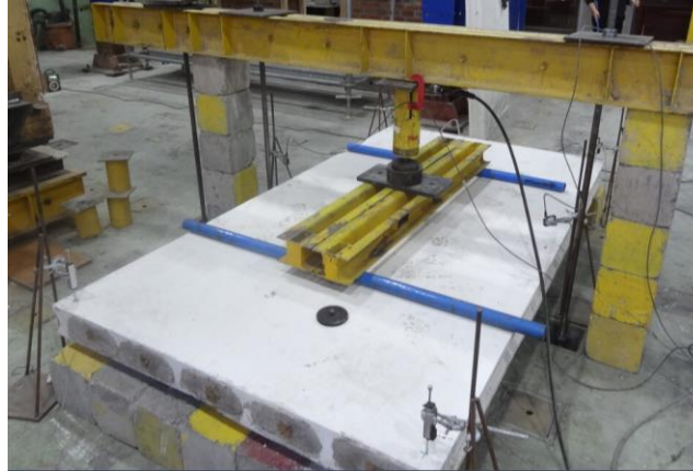
Photograph 7.3.1.1. setup and instrumentation of the bending test.
