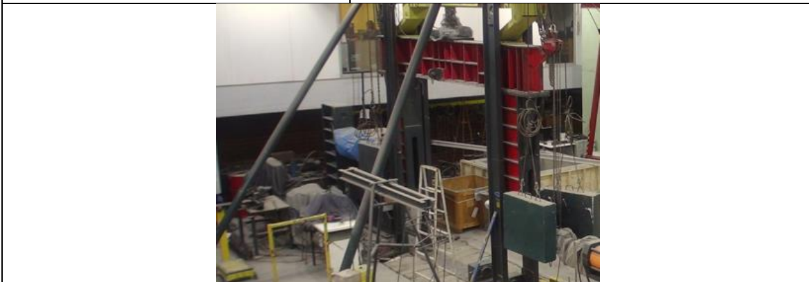
Photograph 7.2.1.3. Equipment used for the horizontal load test.
