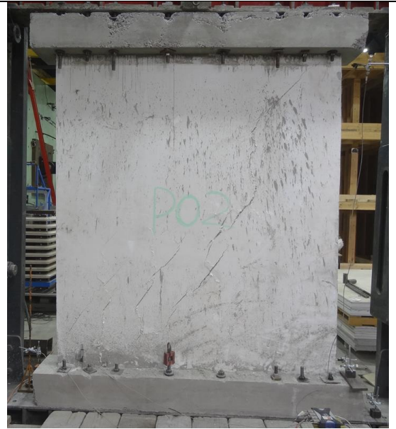
Photograph 7.2.2.2. Typical shear failure in test sample HL-UO-02. Diagonal cracks are observed.
