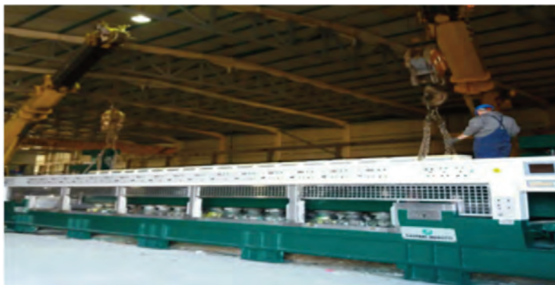
External gantry crane, polishing line being installed and gang saw
