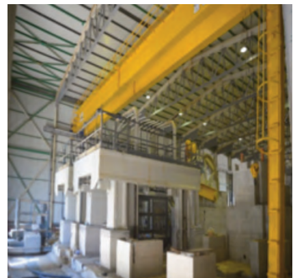
External gantry crane, polishing line being installed and gang saw
