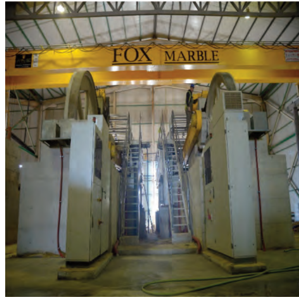
The first block cut at Lipjan, December 2016, and first two gang saws
